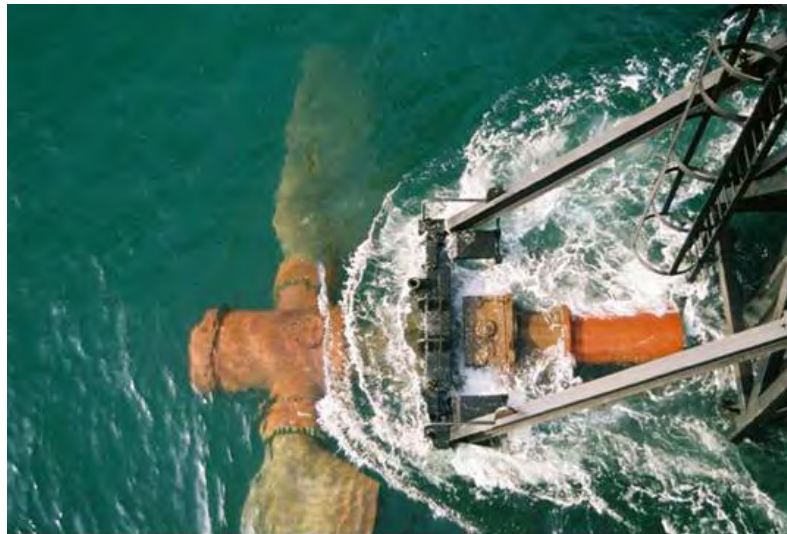
Figure 10. MCT's "Seaflow" tidal stream turbine (brought near surface for maintenance)
